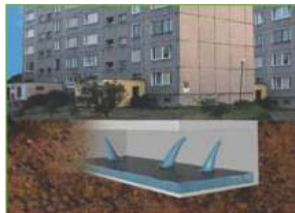
Basements often cannot be accessed from the outside. Thus they can only be waterproofed from the inside (negative side).
